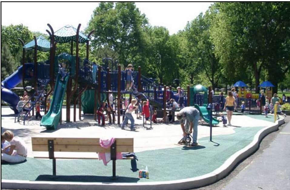
Large playground structure with unitary surface contained by concrete curb perimeter.
