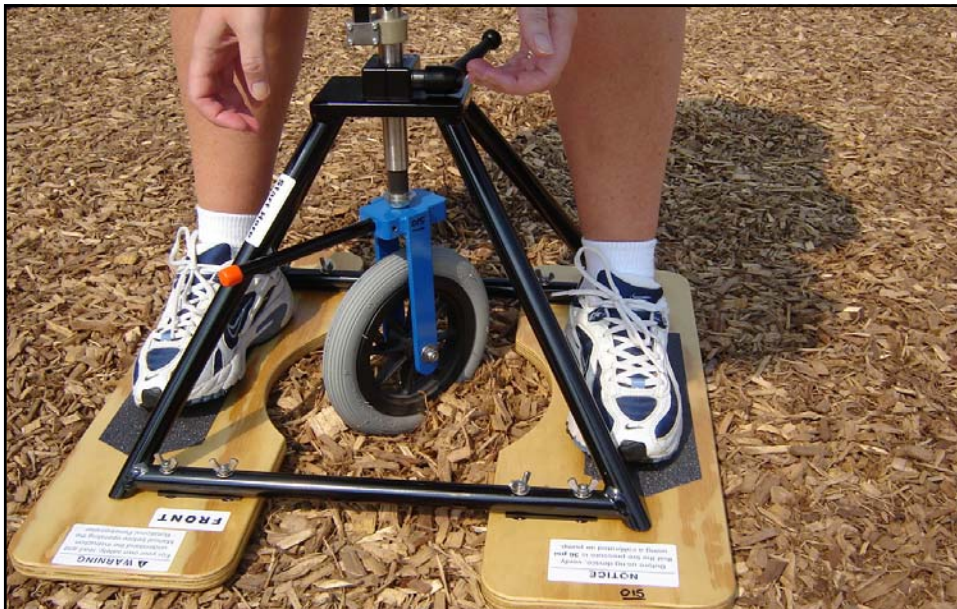
The Rotational Penetrometer. A wheelchair caster on a spring loaded caliber is mounted on a metal tripod with plywood base.
